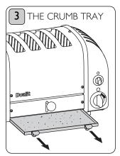
Empty the 'crumb tray' on a regular basis. Daily if being used in a commercial kitchen.
